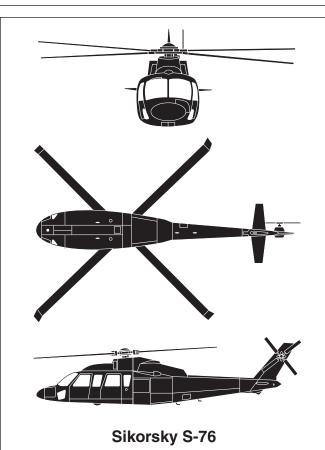
The Sikorsky S-76 first flew in 1977. The S-76A is configured to accommodate 12 passengers and two pilots. It has a maximum takeoff weight of 10,300 pounds (4,672 kilograms), a maximum cruising speed of 145 knots and a service ceiling of 15,000 feet. The S-76A has a maximum range of 404 nautical miles (748 kilometers) with 12 passengers, standard fuel and 30-minute reserves. The S-76A is powered by two Allison 250-C30 turboshaft engines, each rated at 650 shaft horsepower (485 kilowatts).◆
