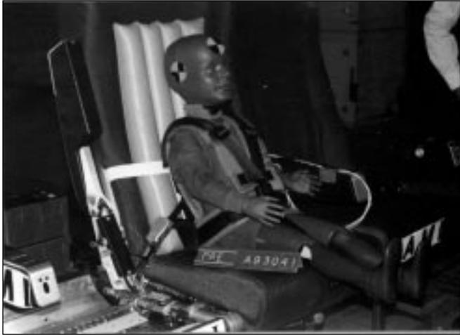
**Figure 2. Three-year-old ATD wearing harness-type restraint device.**
