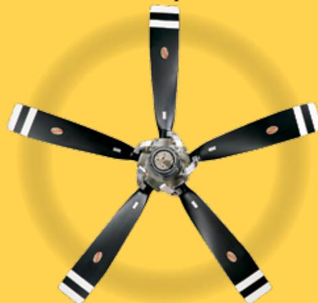
speeds of 1,000 to 1,200 revolutions per minute (rpm), propeller tip speeds are 200 to 300 mph (322 to 483 kph) or more.<sup>2</sup>
